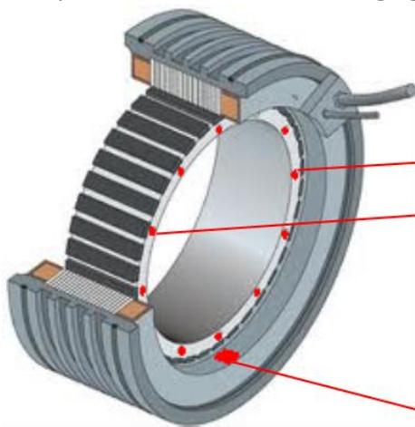
Temperature sensor tags distributed in the rotor
