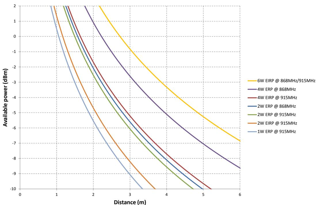
Figure 3: Available power for different regulatory conditions.
