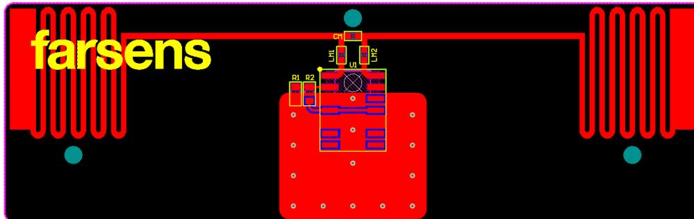
Figure 1: Layout of MKS antenna for ANDY100 with S14 package.
