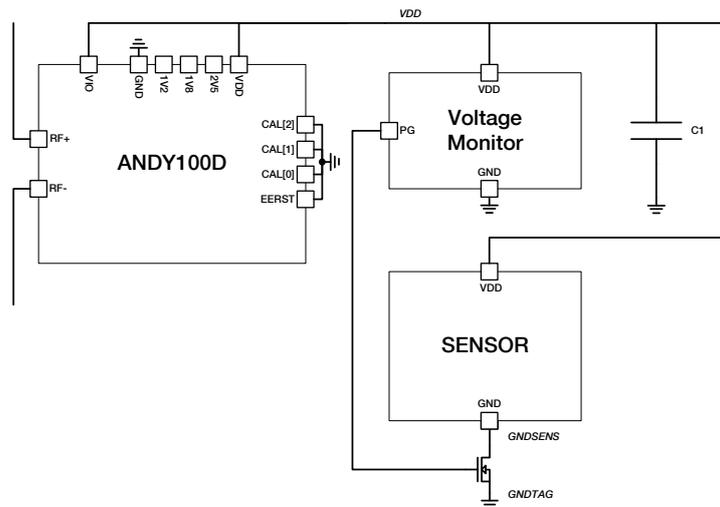
For example, the MAX6427MR IC of Maxim can be used to connect the sensor once the supply voltage is above 2.4V, and disconnect it when the supply voltage falls below 1.8V. In this example, the energy available for the initialization of the sensor is
